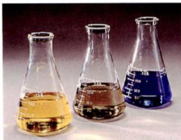
Figure 19.6 The color change of the indicator bromthymol blue. The acidic form of bromthymol blue is yellow ( left ) and the basic form is blue ( right ). Over the pH range in which the indicator is changing, both forms are present, so the mixture appears greenish ( center ).
